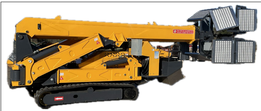
Folded – Self-Propelled Mode or for transportation
